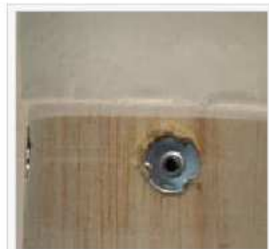
T-nuts in the nose cone retain the payload section.
